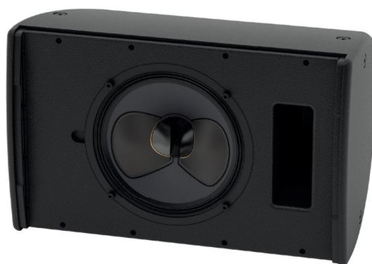
The CDD10 is a very compact two-way passive loudspeaker system which utilises a 10" (250mm) LF/1" (25mm) exit HF Coaxial Differential Dispersion driver. It is uniquely placed to meet the foreground requirements of music bars and clubs, as well as the varied architectural applications that require upfront sound levels from a very compact enclosure. Use with a CSX118 or CSX218 subwoofer will enable the CDD10 to operate as small dancefloor system that is remarkably powerful for its size.
